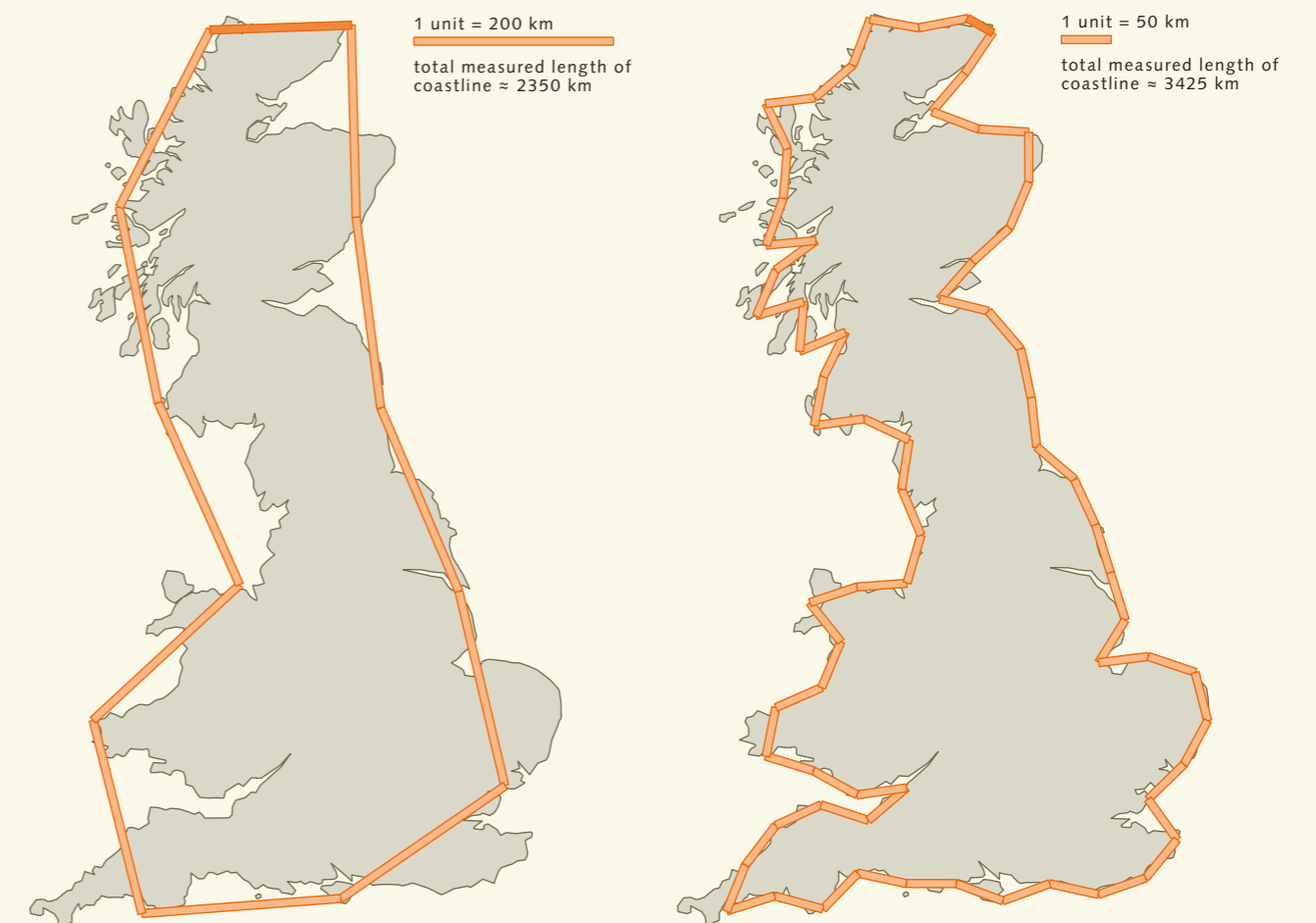
1.18 > The finer the scale used to measure a coastline, the greater the calculated length becomes.
